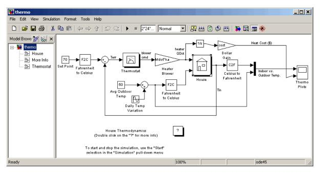
It also creates a scope window for the model. The Scope block displays two plots labeled Indoor vs. Outdoor Temp and Heat Cost (\$), respectively.
