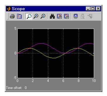
The simulation stops when it reaches the stop time specified in the **Configuration Parameters** dialog box or when you choose **Stop** from the **Simulation** menu or click the **Stop** button on the model window's toolbar (Windows only).
