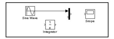
If you look again at the model at the beginning of this section, you'll notice that most of the lines connect output ports of blocks to input ports of other blocks. However, one line connects a *line* to the input port of another block. This line, called a *branch line*, connects the Sine Wave output to the Integrator block, and carries the same signal that passes from the Sine Wave block to the Mux block.
