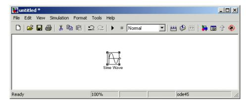
Copy the rest of the blocks in a similar manner from their respective libraries into the model window. You can move a block from one place in the model window to another by dragging the block. You can move a block a short distance by selecting the block, then pressing the arrow keys.
