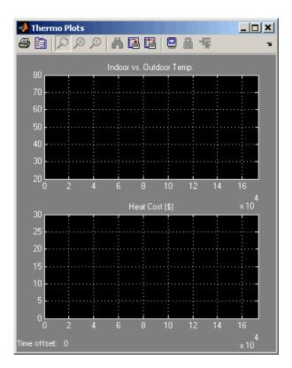
**3** To start the simulation, pull down the **Simulation** menu and choose the **Start** command (or, on Microsoft Windows, click the **Start** button on the Simulink toolbar). As the simulation runs, the indoor and outdoor temperatures appear in the Indoor vs. Outdoor Temp plot as yellow and magenta signals, respectively. The cumulative heating cost appears in the Heat Cost (\$) plot.
