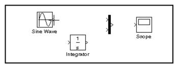
Hold down the mouse button and move the cursor to the top input port of the Mux block.
